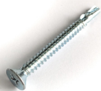
(e) 4.8 x 32mm Csunk Self-drilling Screw Skirt to edge beam
